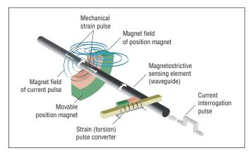
Fig. 1: Time-based magnetostrictive position sensing principle
