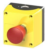
ENCLOSURE FOR COMMAND DEVICES, 22MM, ROUND, ENCLOSURE MATERIAL METAL, ENCLOSURE TOP PART YELLOW, 1 COMMAND POSITION, A=EMERG. STOP MUSHR. PUSHBUTTON RED, 40MM, ROTATE-TO-UNLATCH, 1NC, SCREW CONNECTION, FLOOR MOUNTING, 1 X M20 EACH AT TOP AND BOTTOM !!! Phased-out product !!! SIRIUS ACT 3SU1 is successor Preferred successor type is >>3SU1851-0NA00-2AA2<<
